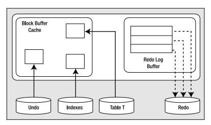
Figure 9-2. State of the system after a redo log buffer flush
