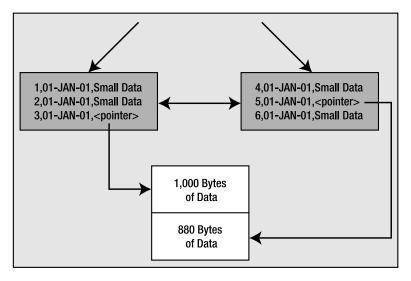
Figure 10-6. IOT with overflow segment, PCTTHRESHOLD clause
