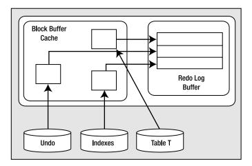
Figure 9-1. State of the system after an INSERT
